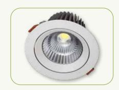
Ceiling cutout: Ø 75 mm, height 62 mm for 8 W. Ceiling cutout: Ø 90 mm, height 75 mm for 12 W Ceiling cutout: Ø 120 mm, height 90 mm for 20 W. Ceiling cutout: Ø 142 mm, height 98 mm for 30 W ORDERING: MODULE (MOD) + DRIVER (DRIVER TO BE ORDERED SEPARATELY)
