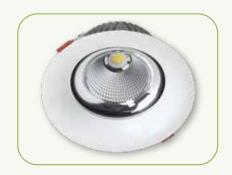
Ceiling cutout: Ø 80 mm, height 50 mm for 8 W. Ceiling cutout: Ø 105 mm, height 65 mm for 12 W Ceiling cutout: Ø 128 mm, height 80 mm for 20 W. Ceiling cutout: Ø 183 mm, height 105 mm for 30 W Ceiling cutout: Ø 205 mm, height 117 mm for 45 W ORDERING: MODULE (MOD) + DRIVER (DRIVER TO BE ORDERED SEPARATELY)
