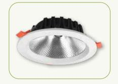
Ceiling cutout: Ø 70 mm, height 40 mm for 8 W. Ceiling cutout: Ø 80 mm, height 41 mm for 12 W Ceiling cutout: Ø 90 mm, height 41 mm for 15 W. Ceiling cutout: Ø 110 mm, height 51 mm for 20 W Ceiling cutout: Ø 160 mm, height 53 mm for 30 W. Ceiling cutout: Ø 190 mm, height 57 mm for 40 W
